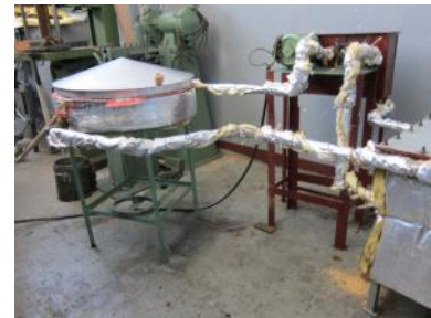
Oil circulation to baking pan (AAU)
