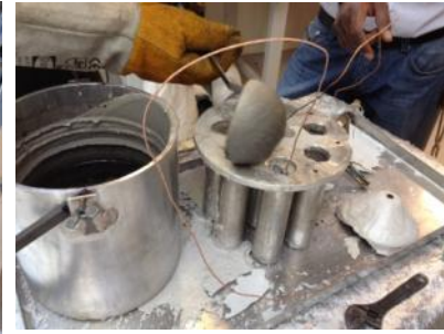
Filling PCM in cylinders
