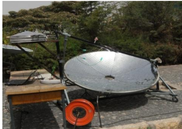
Steam generation and coupling to baking pan (Mekelle)
