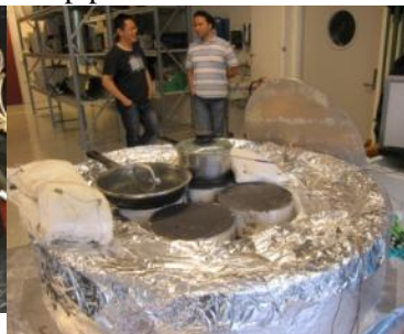
Assembly of four PCM containers (NTNU)
