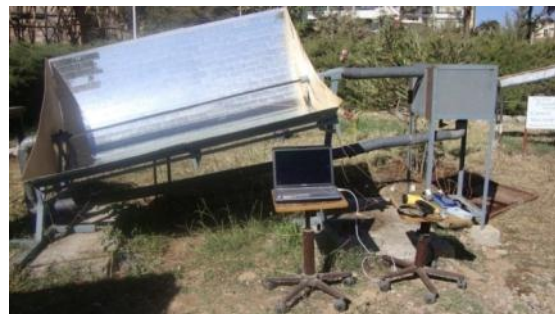
Trough with Oil/PCM storage (Mekelle)
