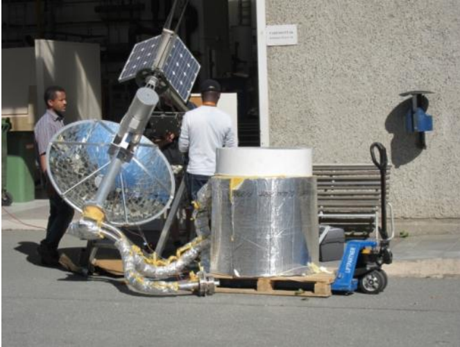
Air/rock bed test
