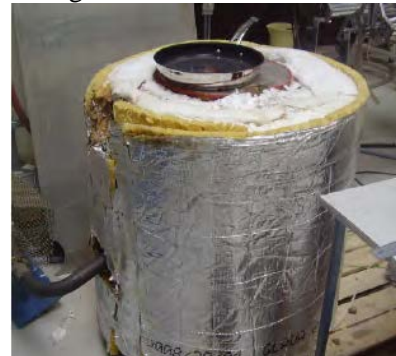
Ceramic insulation rock bed
